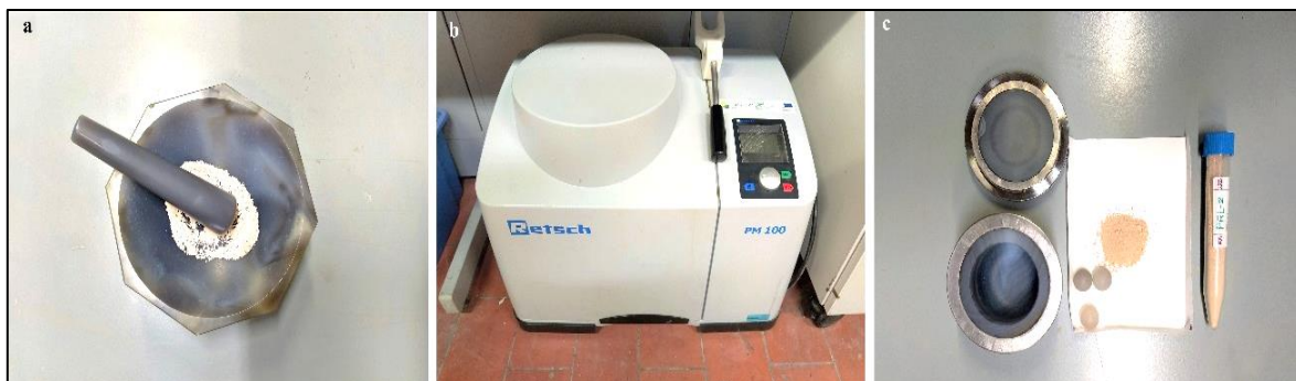
Figure 3. 5- Tools used for the preparation of the powdered samples: a) Disaggregation by mortar and pestle, b) Powdering equipment PM 100 Planetary Ball Mill (Retsch), c) Agate grinding jar and grinding balls
