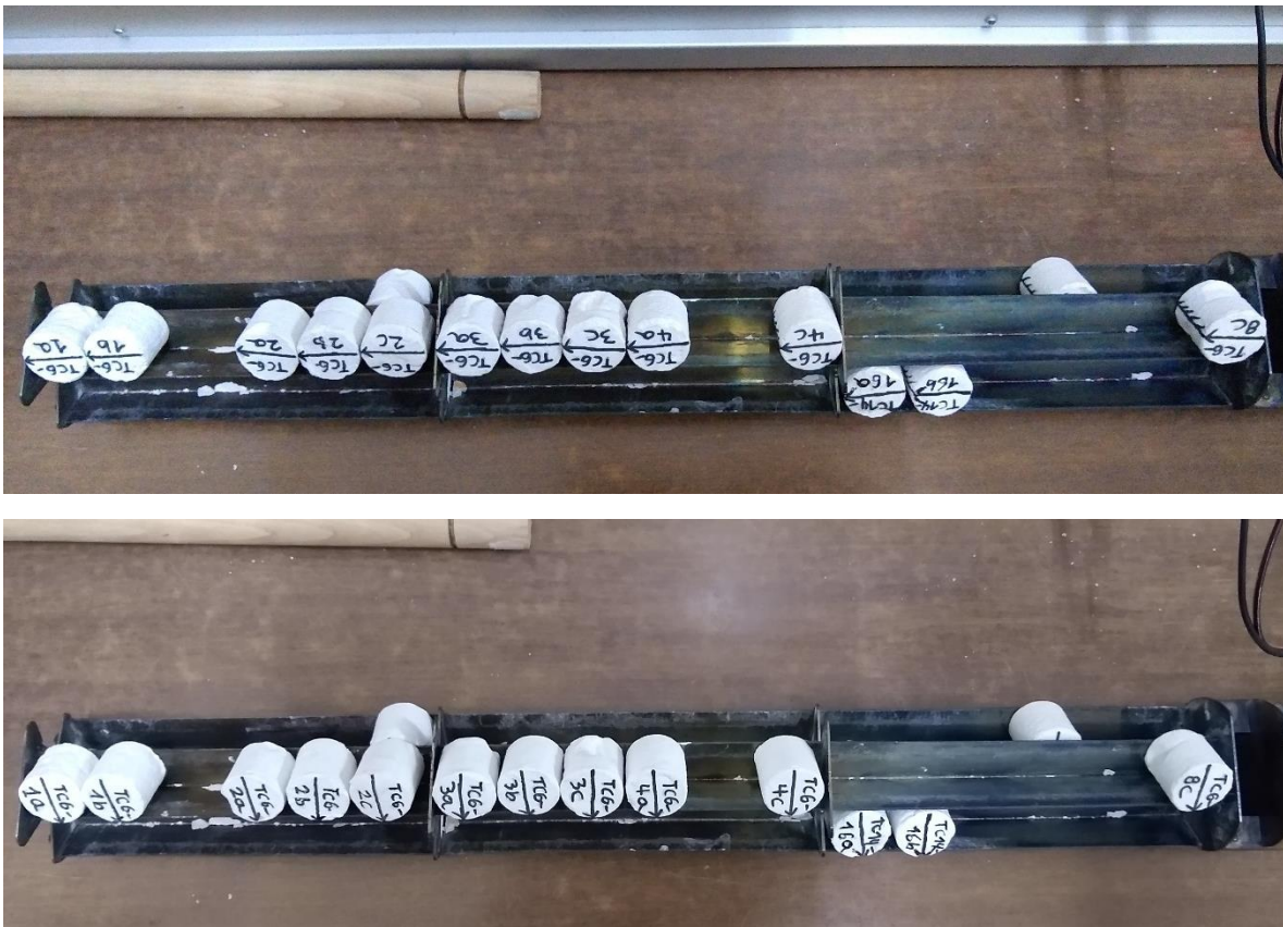
Figure 12 - Alignment of the specimens on their X axis (top) and Y axis (bottom). They are heated and then cooled in this position, in contrast to the main Z axis.
