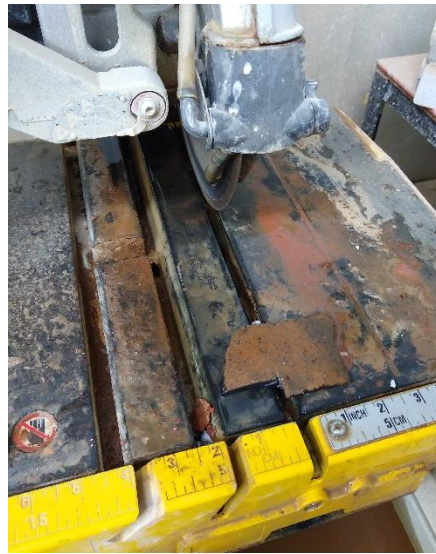
Figure 8 - Workshop saw used to cut the samples into the specimens
