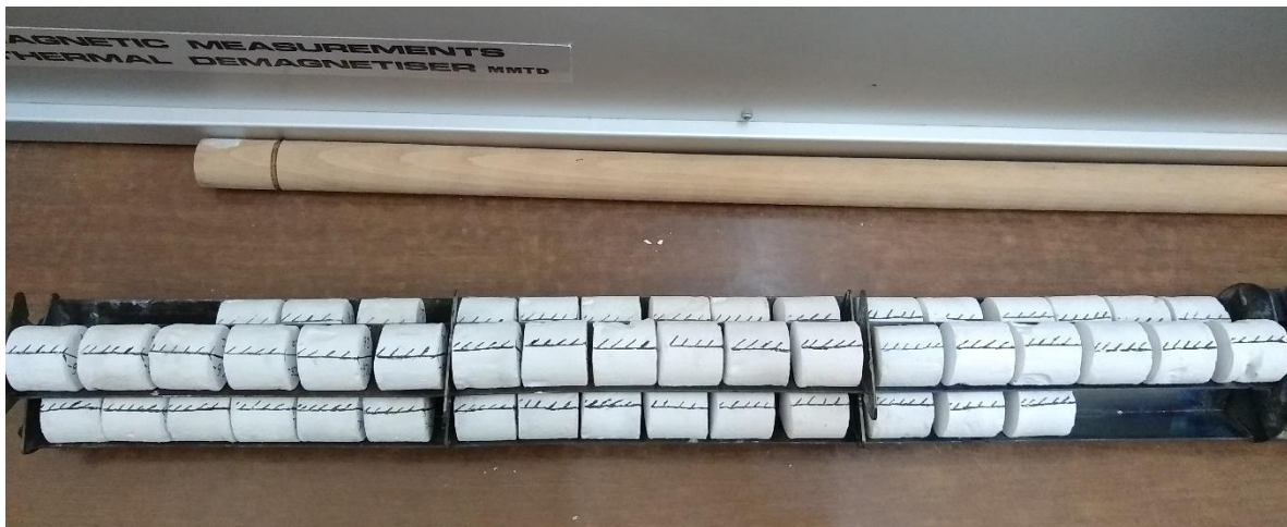
Figure 10 - Specimens aligned before a heating/cooling cycle of the Thellier-Thellier method. The guidelines help to maintain the same order which is important for the field applied.
