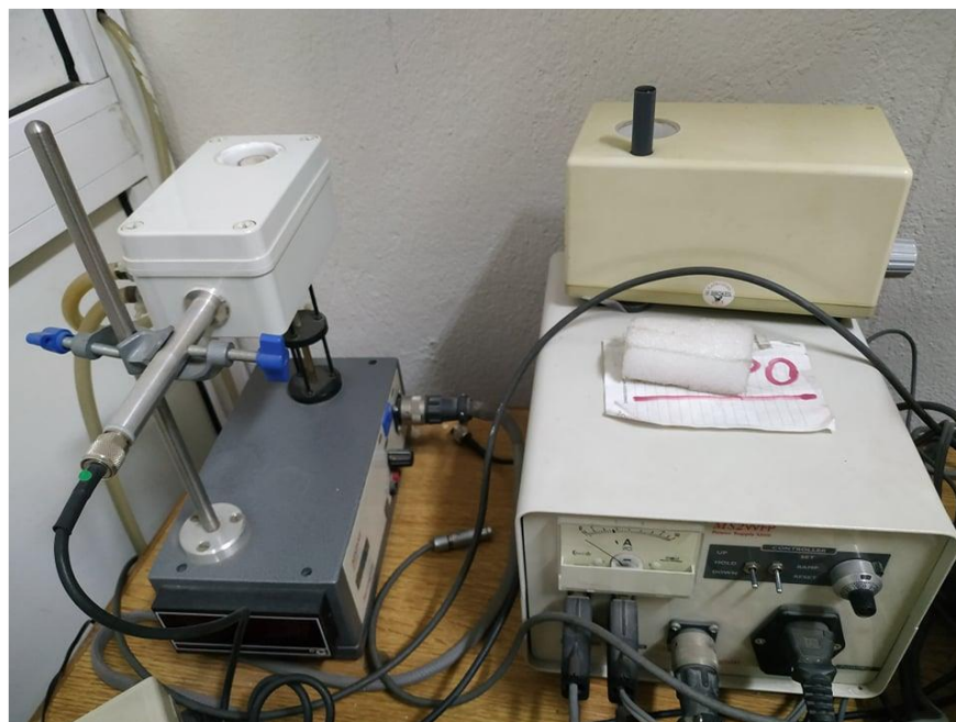
Figure 15 - Models MS2WFP of Furnace (left) and Power Supply Unix (right), by Bartington Instruments
