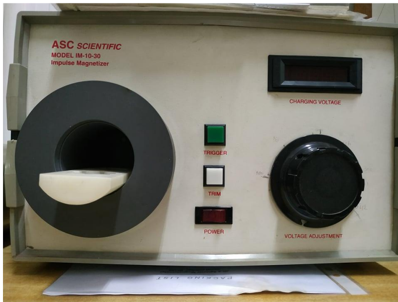
Figure 17 - ASC Scientific IM-10-30 Impulse Magnetizer, Bartington Instruments
