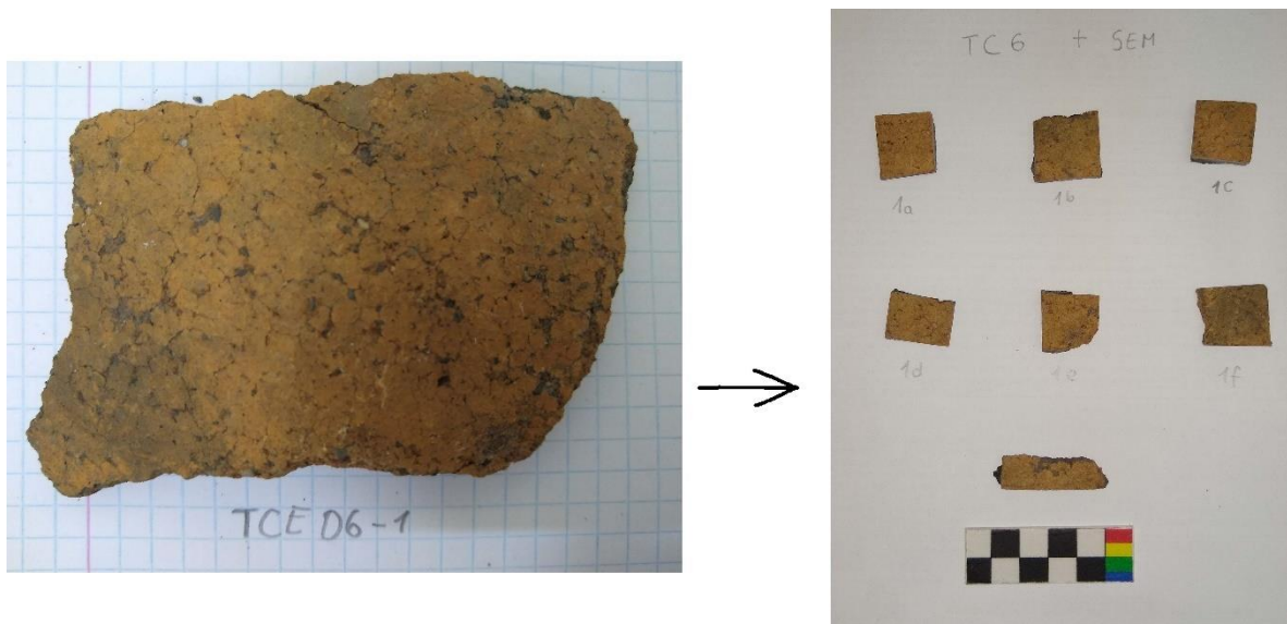
Figure 7 - From the original sample to the specimens (with the cut for petrographic analysis)
