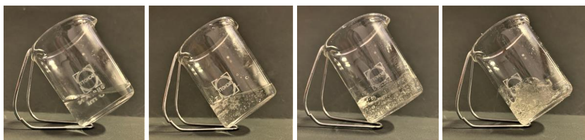
Figure 3.3. Pictures of the gel based on CMC with different concentrations.
