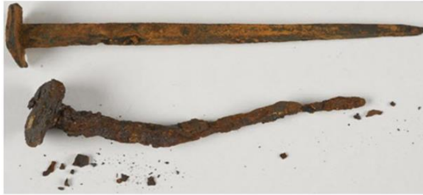
Figure 1.1 Examples of stable (top) and active (bottom) corrosion on copper nails. Government of Canada, Canadian Conservation Institute.
