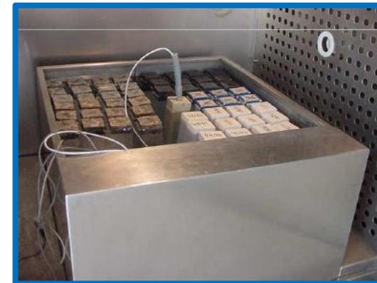
Implications of exposure to high temperatures for stone cladding requirements of three Portuguese granites regarding the use of dowel-hole anchoring systems
