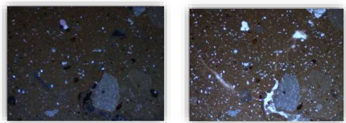
Figure 36 Optical light microscope images of sample TFN.1954.B. 272/5 in PPL (left) and XPL (right).
