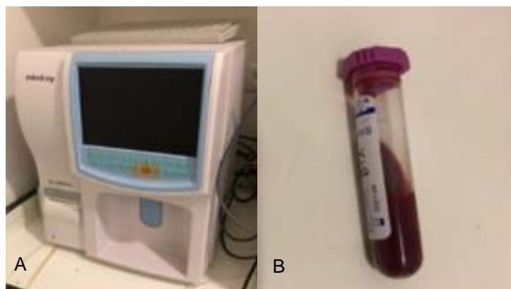
Figure 6—Equipment used to perform the CBC in the population; A- hematology analyzer; B- EDTA tube with blood (original image)
