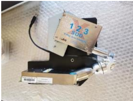
Fig. 6 X-ray source and detector
