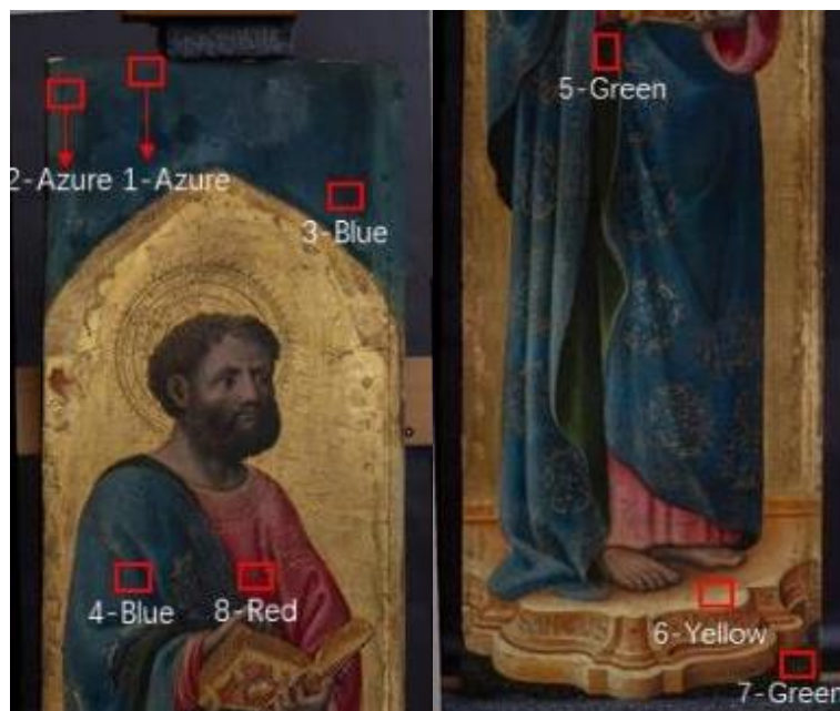
Fig. 92 XRF test points in St. Mark
