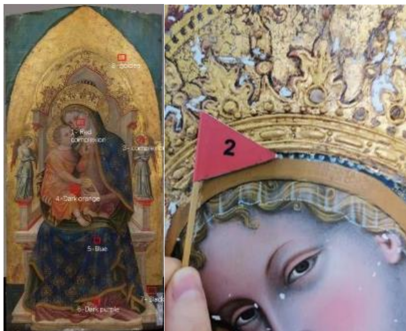
Fig. 107 XRF test points in the Virgin to the throne and the child
