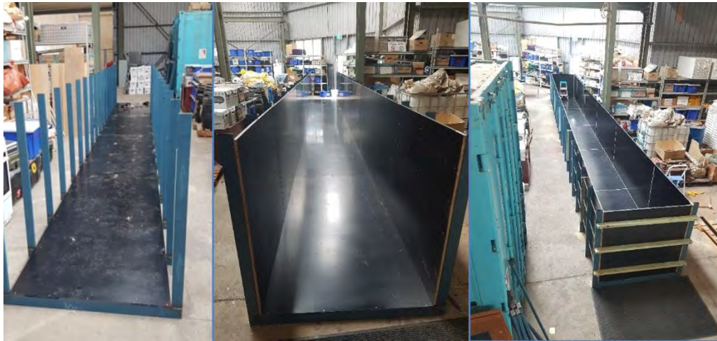
Figure 6: 12m test tank as built at various stages of the build
