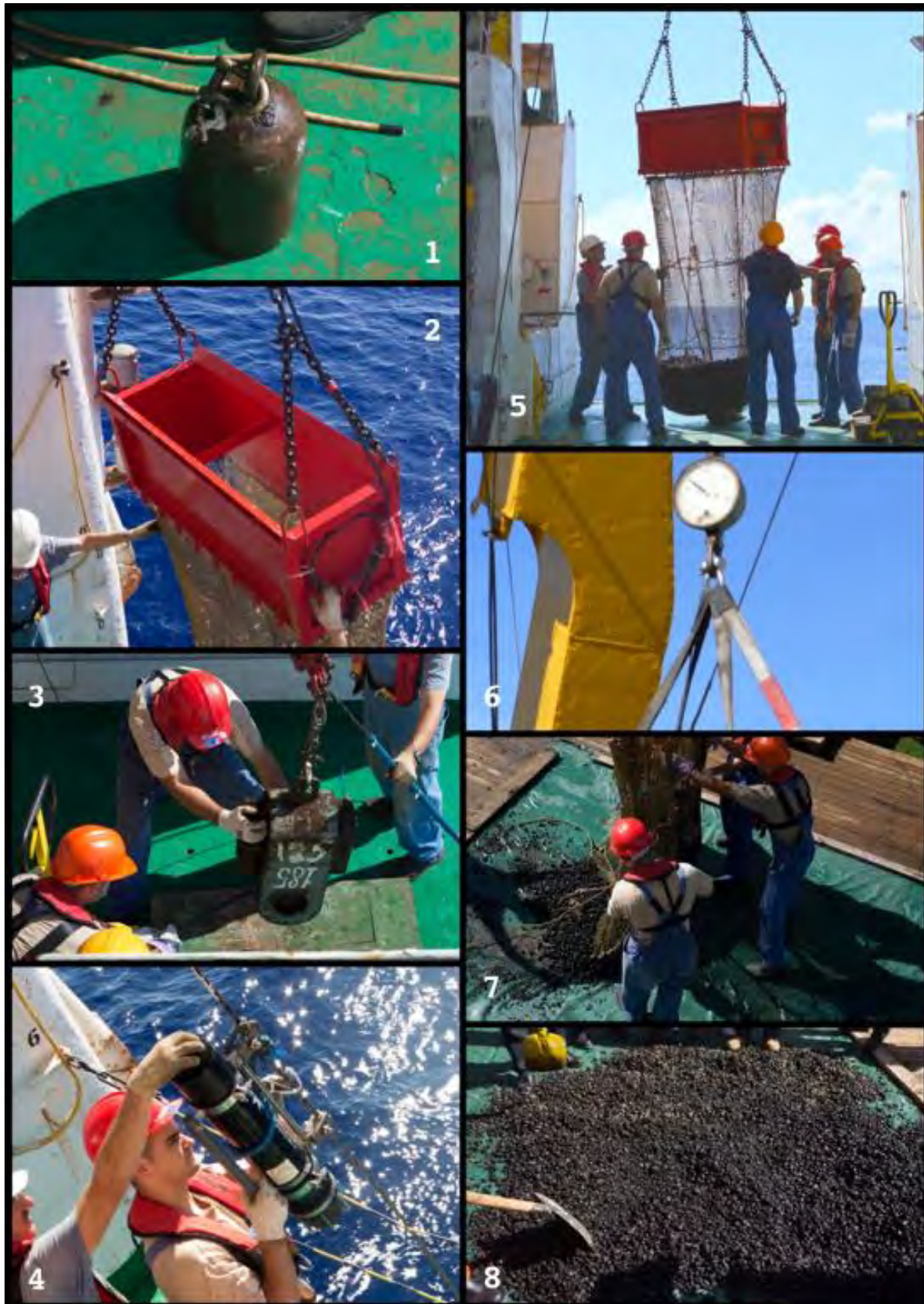
Figure 4-7: Operations and details of the YMG Galatea-trawl dredge
