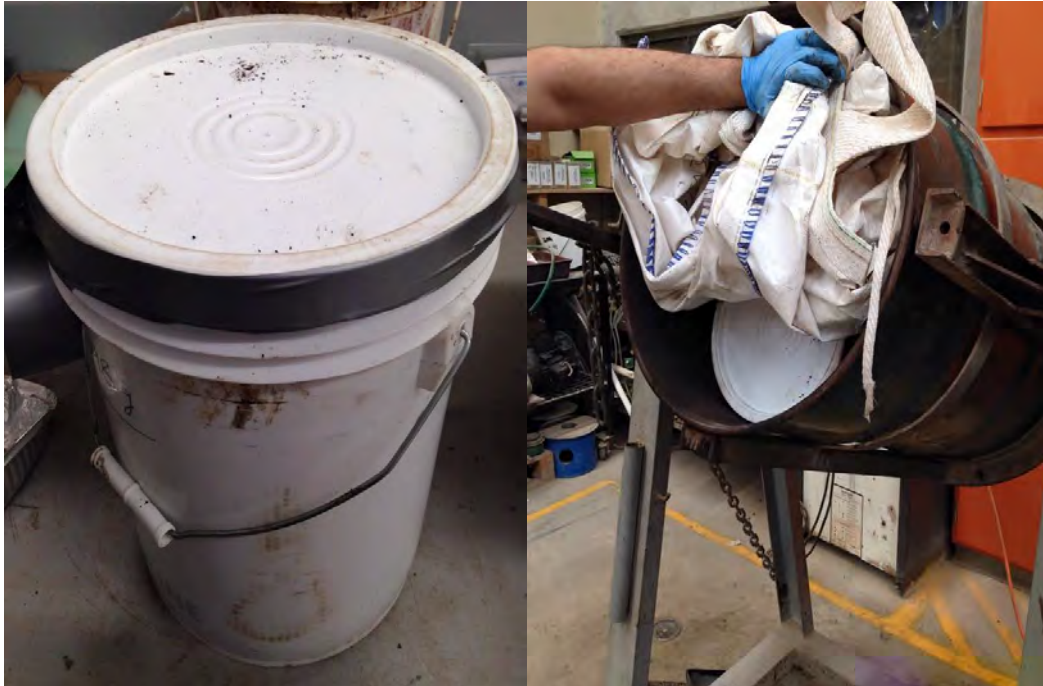
Figure 4-79: Wet sample bucket held in place with crates/padding and sealed with tape.
