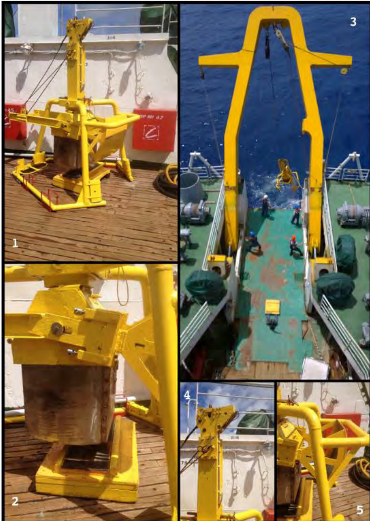
Figure 4-11: Details and recovery of the YMG box-corer
