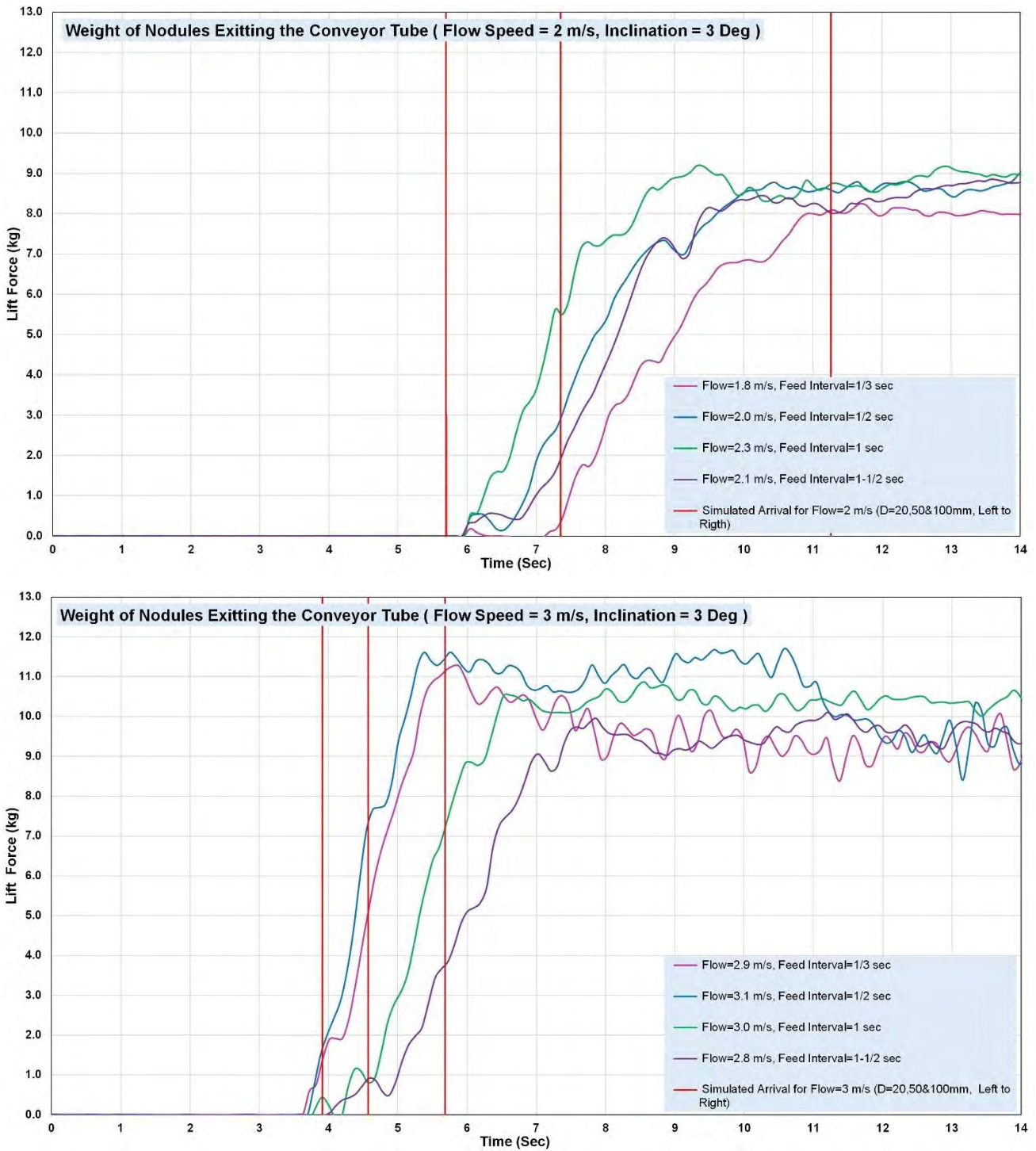
Figure 22: Time History of Weight of Nodule Particles Exiting the 6 m Conveyor with an Inclination of 3° : For Flow Velocities = 2 and 3 m/s (Top and Bottom)
