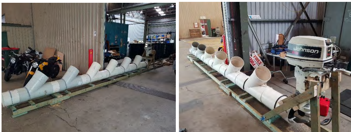
Figure 7: 300 mm x 6m conveyor as built, “Ts” are spaced 1m apart
