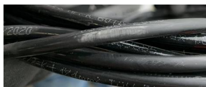
Figure 8: Cable 2 (saltwater tank) showing signs of physical degradation of the insulation layer.
