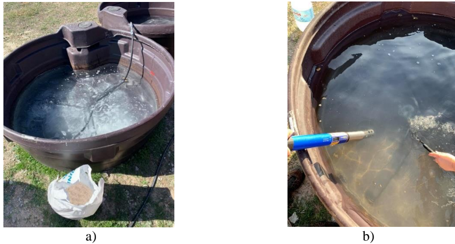
Figure 4 a) Preparation of saltwater; b) Physical-chemical characterization with the multiparametric probe
