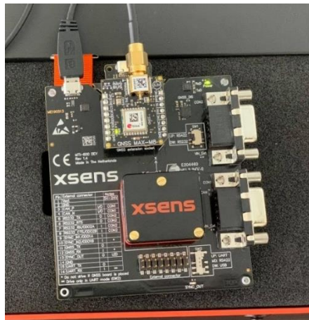
Figura 22. Sensor inercial MTi-670-DK
