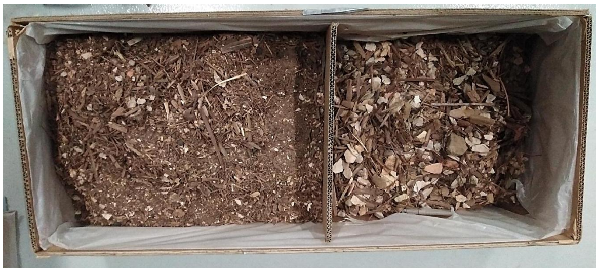
Figure 12. The box divided into two parts, the large part contain the “original material” and the second part the coarser pieces like wood pieces, stones and plant branches (photo: NagmEldeen 2020).
