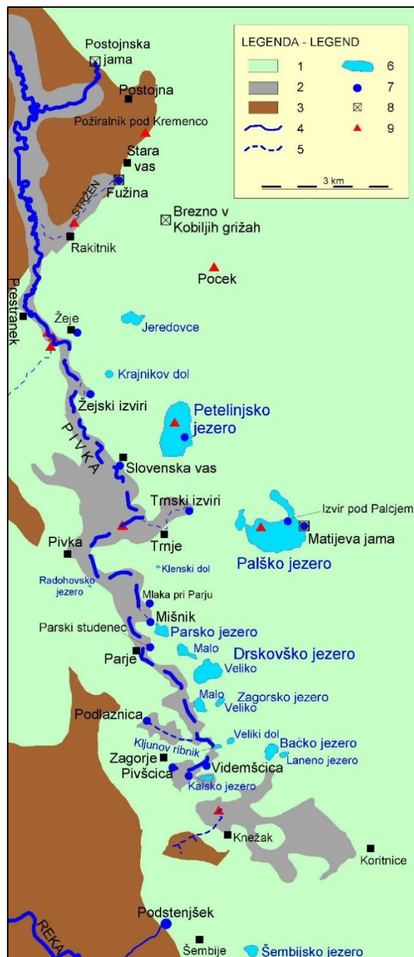
Fig. 2.02: Hydrogeological map of the Pivka Valley (Petrič & Kogovšek 2005). Legend: 1. Karst aquifer, 2. Porous aquifer, 3. Very low permeable rocks, 4. Surface flow, 5. Intermittent surface flow, 6. Intermittent lake, 7. Major spring, 8. Water cave, 9. Injection point.
