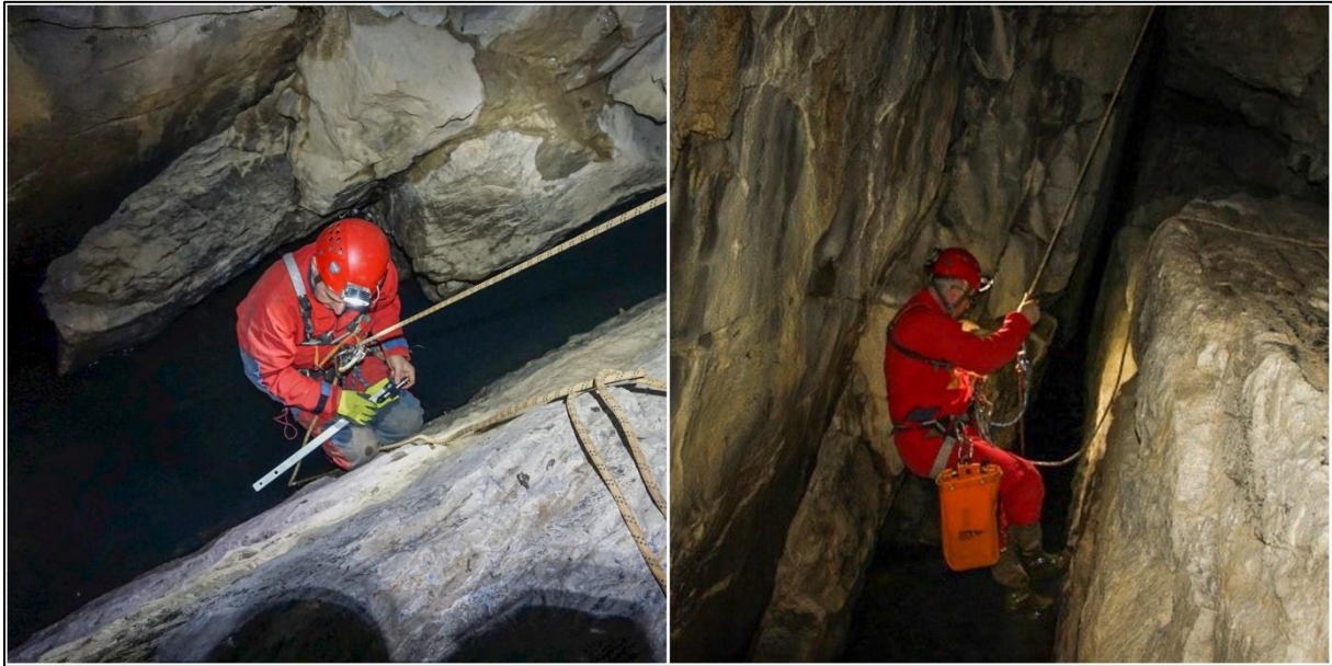
Figure 1.04: Placement of water level, temperature and conductivity data loggers in the Jama/Antro di Bagnoli spring.
