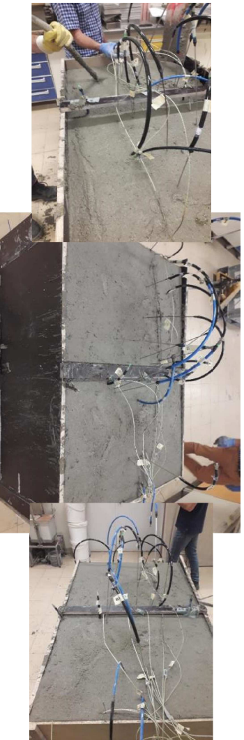
Figure 6.1.4. Module core construction. OPC + Fly ash concrete appearance
