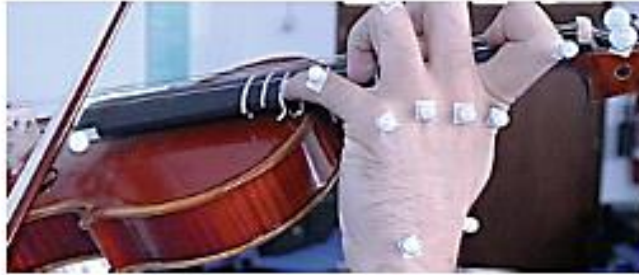
Image 2. Reflectors placed on the metacarpophalangeal joints, and at the four extremities of the violin fingerboard
