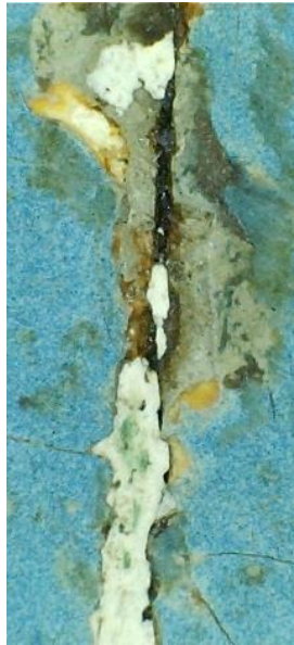
Fig.14. Microscopic photography showing the different intervention layers around the right crack
