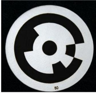
Figura 7 - RAD - Ring Automated Detected - alvo do PhotoModeler UAS. Fonte: <https://www.photomodeler.com>.
