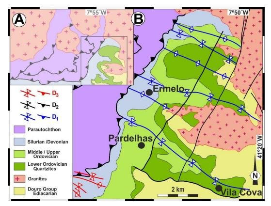
**Figure 7** – General structural map northern of Marão Mountain showing the interference between  $D_1$  and  $D_3$  folds with  $D_2$  thrusts (adapted from Pereira, 1989).
