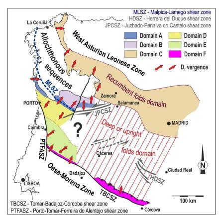
**Figure 4** – Main fold pattern in the CIZ of NW Iberia (adapted from Azor *et al.*, 1994; Díez Balda *et al.*, 1990; Ribeiro *et al.*, 1990; Dias and Ribeiro, 1994; Dias, 1998; Dias *et al.*, 2013b; Romão *et al.*, 2013).
