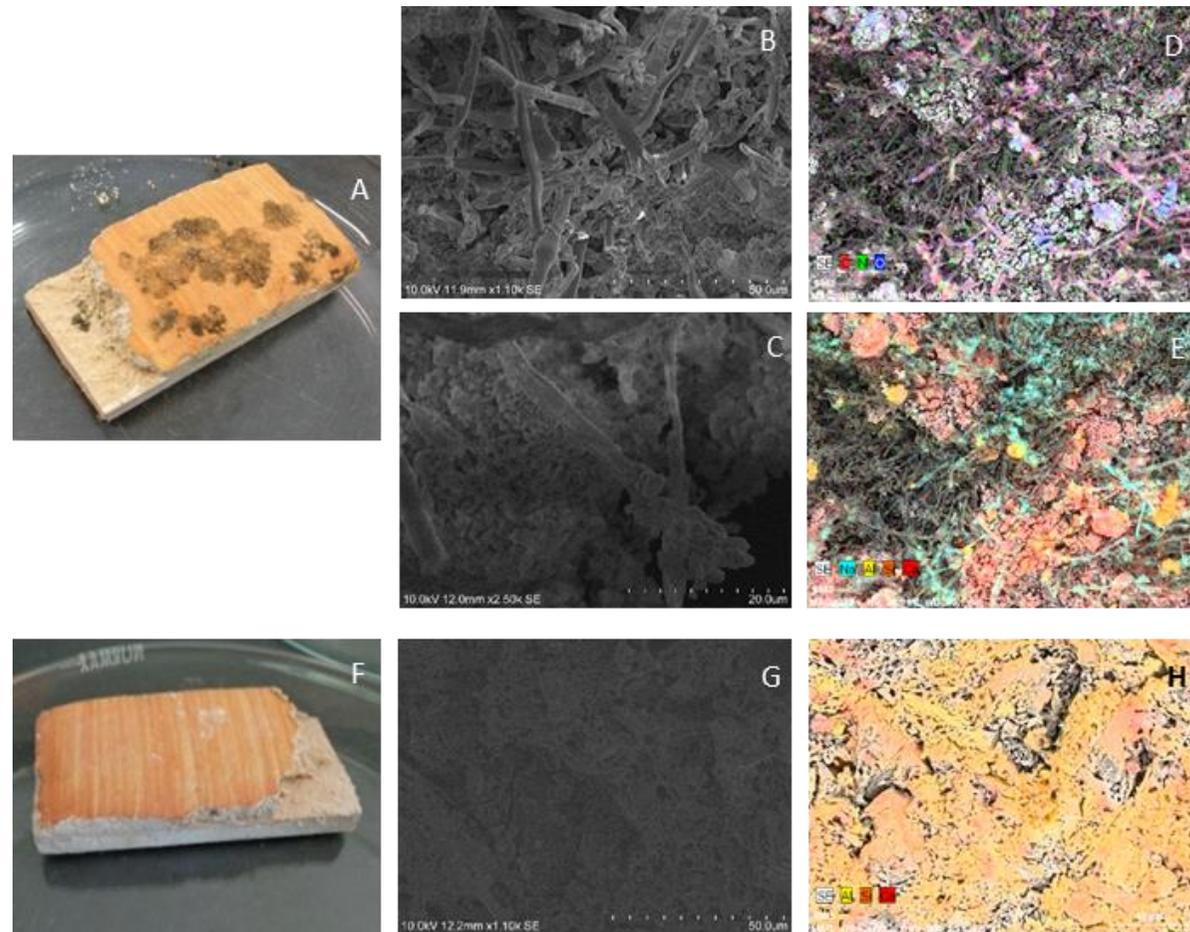
Figure V-5: Mortar slabs, SEM micrographs of the MS1 microfragments and EDS analysis. A-E: control slabs inoculated with *Cladosporium* sp.; F-H: MS with CB 3 (bioactive compounds produced by *Bacillus* sp. CCLBH 1053).
