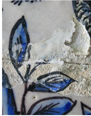
Figure 9. Detachment of the glaze in the surrounding area of the lacuna.
