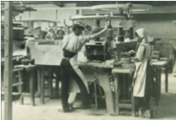
Image A.129 - tile making by hand pressing
