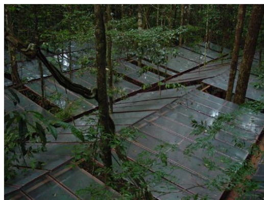
Figure 1. Infrastructure of Through-fall Exclusion experiment installed over 100x100 m plot at Caxiuanã.
