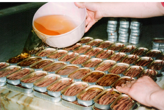
Figure 5 – Oil covers the fish completely, with minimum spillage
