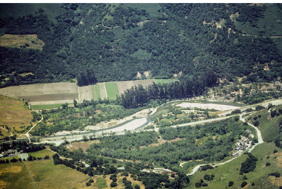
Figure 2 – Aerial view of the Carmel River, California, showing a meander bend cut off by the Monterey County Public Works Department to straighten the road in the 1960s (bottom of photo). In the subsequent years, the river eroded a sympathetic meander bend to the south (top of photo) to compensate for the loss of sinuosity. (Photo by author, 1983)
