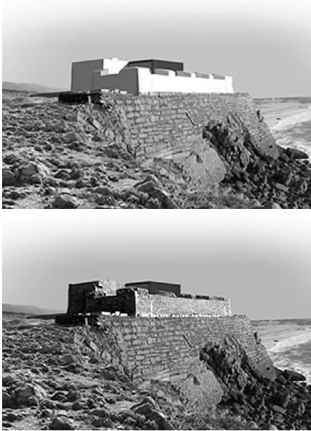
Figure 4 – Three-dimensional simulation: fort walls with and without plaster
