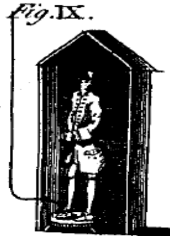
Figure 1.2 Benjamin’s experiment proposal to check cloud electrification, ( Experiments and Observations on Electricity, Made at Philadelphia in America ).
