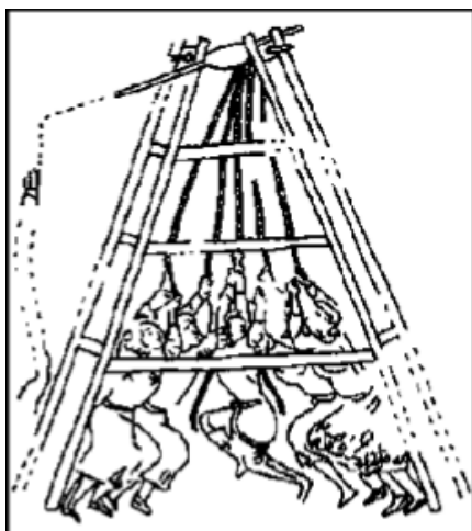
Figura 15 – Gravura do engenho neurobalístico, datado de 1044. (NEEDHAM, J, HAYES, D. D., Science & Civilization in China , Vol. V:6 – Military Technology: Missiles and Sieges, Cambridge University Press, 1994.)
