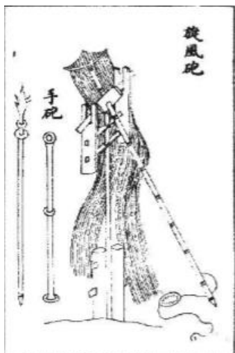
Figura 14 – Gravura de um Phao Chhê , engenho neurobalístico datado de 759. (NEEDHAM, J, HAYES, D. D., Science & Civilization in China , Vol. V.6 – Military Technology: Missiles and Sieges, Cambridge University Press, 1994.)
